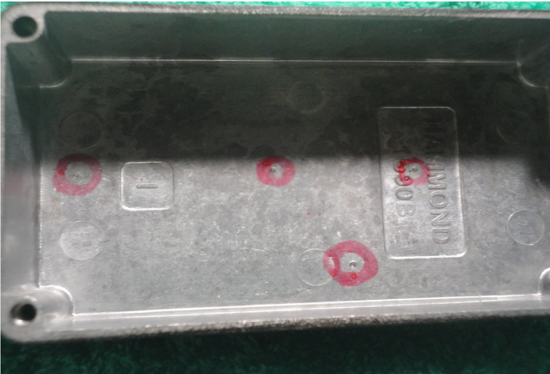
Hole locations are pre centerpunched with a jig.
