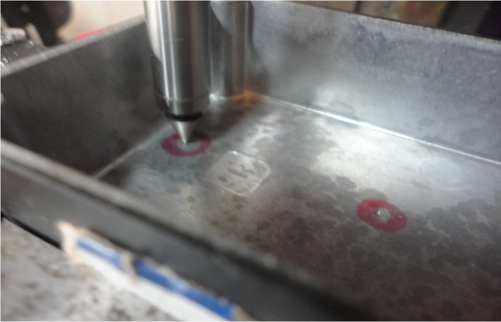
Lining up a hole with a center finder.
